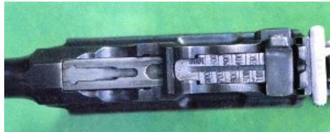
**Sighting equipment consisted of a front blade and a tangent rear, optimistically calibrated out to 1000 meters! The Mauser "barleycorn" sights gave a poor sight picture.**
